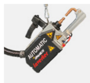
TRANSFORMER Installed inside the gun
